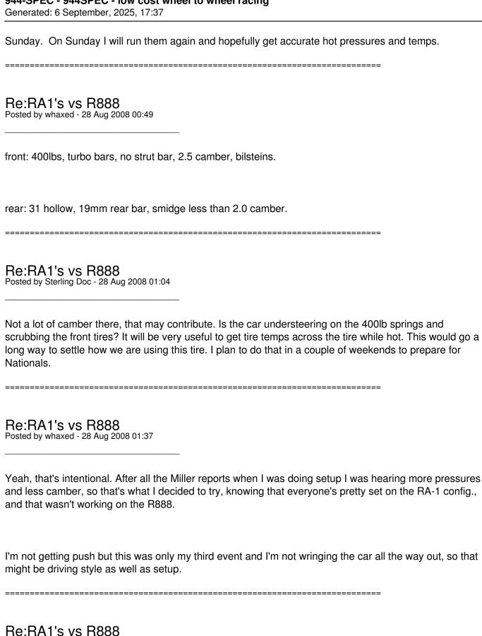
The word from Toyo was the R888 need less camber. Well running over the sidewall is a sign of too little camber. I think for our suspenions we keep the camber the same bump up the pressure.
