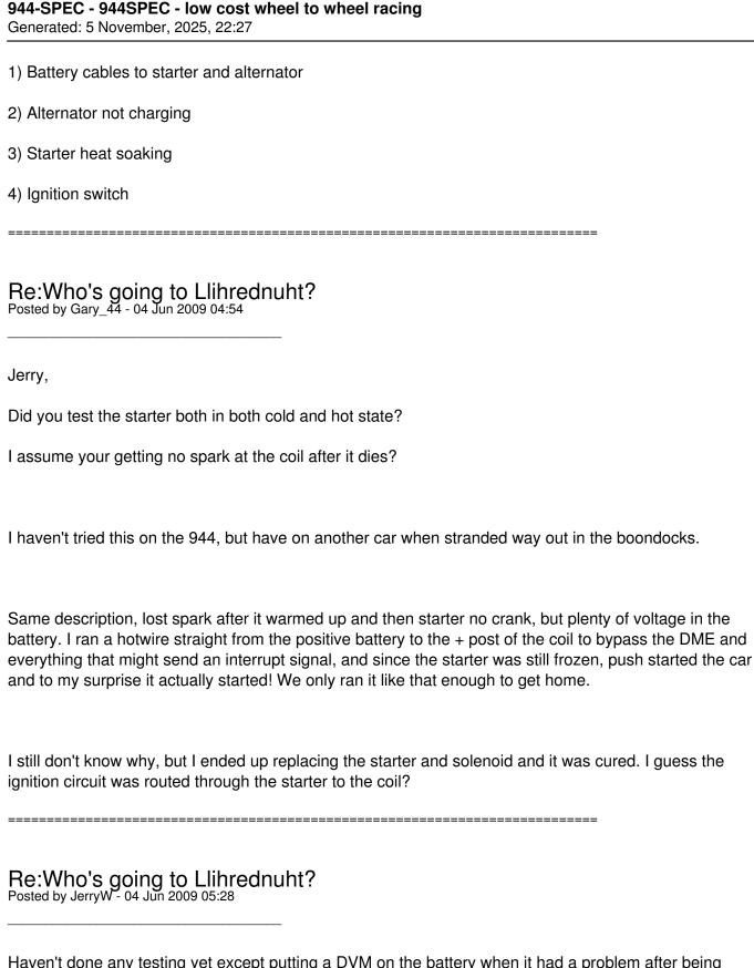
Haven't done any testing yet except putting a DVM on the battery when it had a problem after being towed in. Strange thing is that adding a jump box allowed it to start. So on Sat after the failure I put a new full size battery in place of the lightweight. Problem happened again on Sunday with the new battery within the day.
